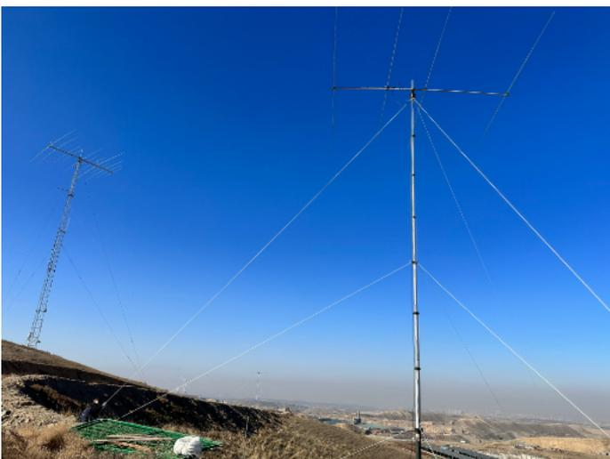
The Optibeam OB12-4 (left) and a 4-Element yagi for 15m (right).
